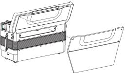
(18) Use the coin to loosen the two screws of the compartment cover.
